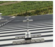
This kit has been carefully designed to allow the installation directly on the metal sheet, to avoid the perforation of the covering layer. Besides, the advantage of having adjustable plates makes it suitable for every possible situation. To avoid oxidation all the components, including bolts are made of stainless steel.
